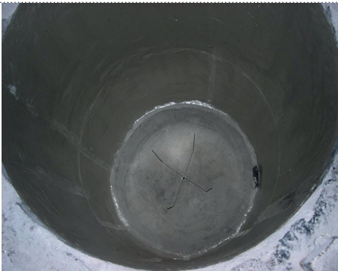
CIF after lining with silica
