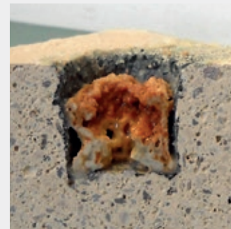
Refractory NOT attacked by alkali
