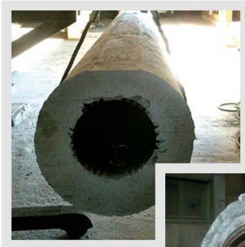
Kiln Burners. Seven Cast corundum.
